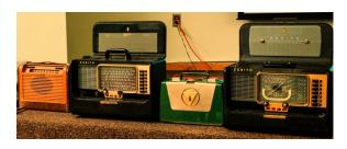
typically used separate so-called "A", "B", and "C" batteries for the vacuum tubes' filament (e.g., 1.5V), plate (e.g., +90V), and grid voltages (e.g. -4.5V), and so had substantial compartments for the batteries.
