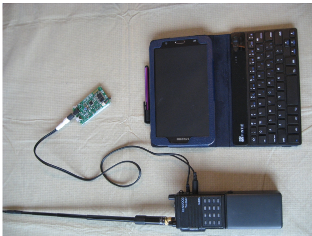
APRS System #2: Mobilinkd TNC1, TH-25AT and Galaxy Tab 5. Some tablets like this one have GPS, the challenge is to input that data into the APRS program.
