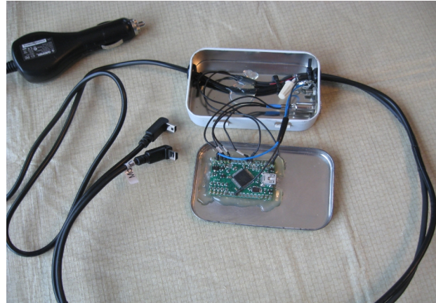
APRS System #1 with box open showing the T3 board and associated wiring. The Garmin nuvi has two USB inputs: one for power and the other for data.
