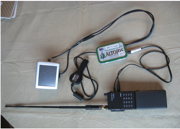
APRS System #1: Garmin GPS (nuvi 350); Argent T3 mini in Altoids box and HT TH-25AT.
