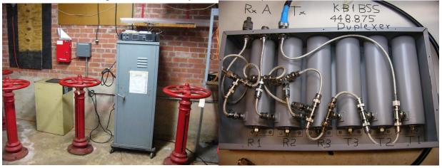
We are not done yet with our upgrades. Currently the 448.875 repeater is using separate antennas for transmitting and receiving. This is the duplexer that was used with the old repeater to allow both the receiver and the transmitter to share the same antenna. We
