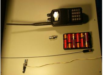
The 1/4 wave antenna is a more efficient radiator of r.f. energy than the factory-supplied rubber duck. The tiger tail is another 1/4 wave wire that can clip onto the ground side of the antenna and dangle down beside the handheld to make an efficient bottom half of a vertical dipole antenna. Older handheld radios universally used rubber ducks with easily connected
