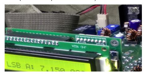
This is a kit, manufactured in India, that uses an Arduino microcontroller to control a frequency synthesizer chip at its heart. It will put out 20 Watts, CW or SSB, on 80 and 40
